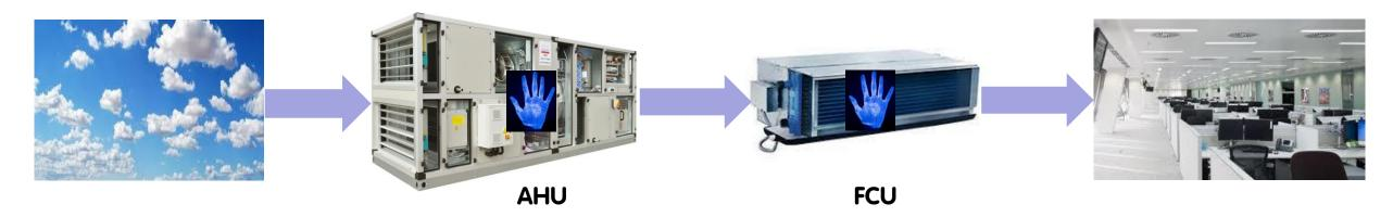
On this journey, the fresh air is filtered in two places. Once within the air handling unit (AHU), and then at the fan coil unit (FCU) before being supplied into the space.
